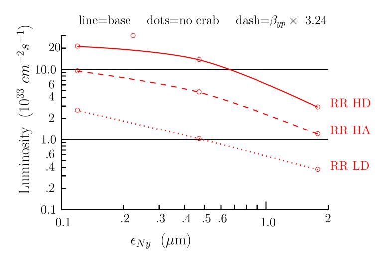
NC) No cooling assuming a  $\epsilon_{Np\perp} = 1.8 \mu \text{m}$ , MC) Moderate cooling with a  $\epsilon_{Np\perp} \approx 0.5 \mu \text{m}$ , and SC) Strong cooling with a  $\epsilon_{Np\perp} \approx 0.12 \mu \text{m}$ .
