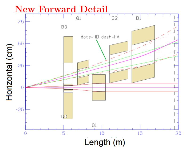
Electron doublet instead of triplet focus Eliminates  $Q_{2e}$  and allows  $B_{1p}$  to move up
