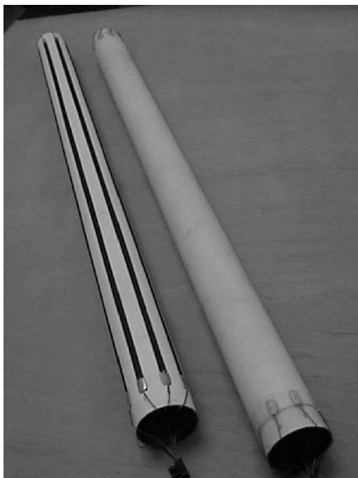
Fig. 4. Tube with plasma sprayed heater strips (left) and with additional alumina insulation (right).
