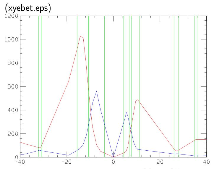
betas are converging to about 150 (x) 80 (y) m at z=27 m and much the same at -33 m in the rear.
