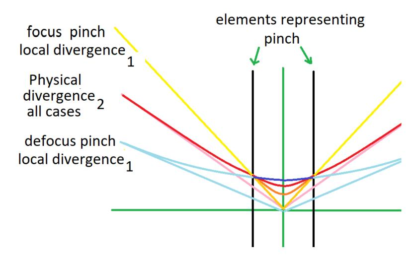
Local focusing (or defocusing) will change the local  $\sigma(IP)$  and also the divergence  $\sigma'(\text{Lattice})$ , increasing it with focus and decreasing it with defocus.
