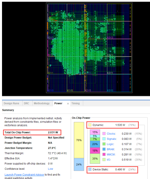
Figure 19 FPGA power estimate.
