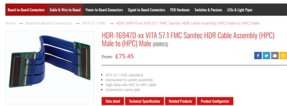
Figure 11 Samtec cable to provide connectivity between a HRPPD_FMC_BOARD.V0 board and a KCU105 kit.
