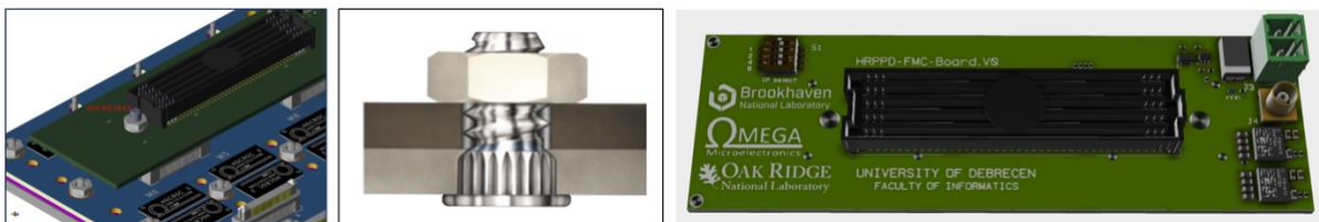
Figure 9 Left: FMC board fixed in situ by KFH studs. One can also see three HV pins on top of the picture and a pair of HRPPD screws on the left. Center: PEM KFH broaching stud (here shown in a configuration without a gap between the two boards). Right: A 3D model of the FMC board. Location of the mechanical holes for broaching studs is indicated by circles on both sides of the HPC connector.
