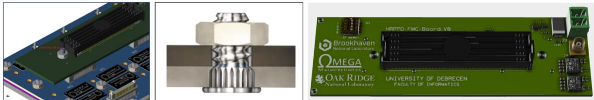
Figure 10 Left: FMC board fixed in situ by KFH studs. One can also see three HV pins on top of the picture and a pair of HRPPD screws on the left. Center: PEM KFH broaching stud (here shown in a configuration without a gap between the two boards). Right: A 3D model of the FMC board. Location of the mechanical holes for broaching studs is indicated by circles on both sides of the HPC connector.
