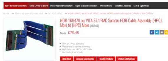
Figure 12 Samtec cable to provide connectivity between a HRPPD_FMC_BOARD.V0 board and a KCU105 kit.
