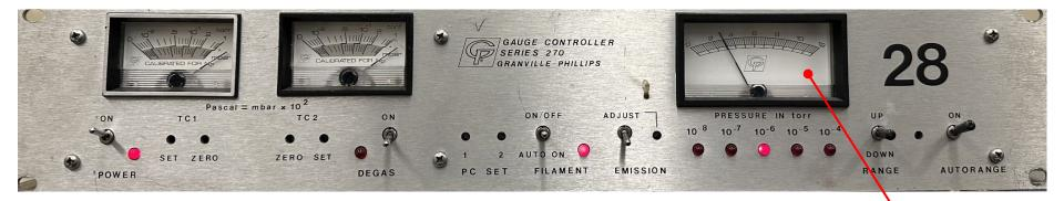
Ionization Gauge: Measure of pressure inside the chamber (~ 3 \* 10^-6 torr )
