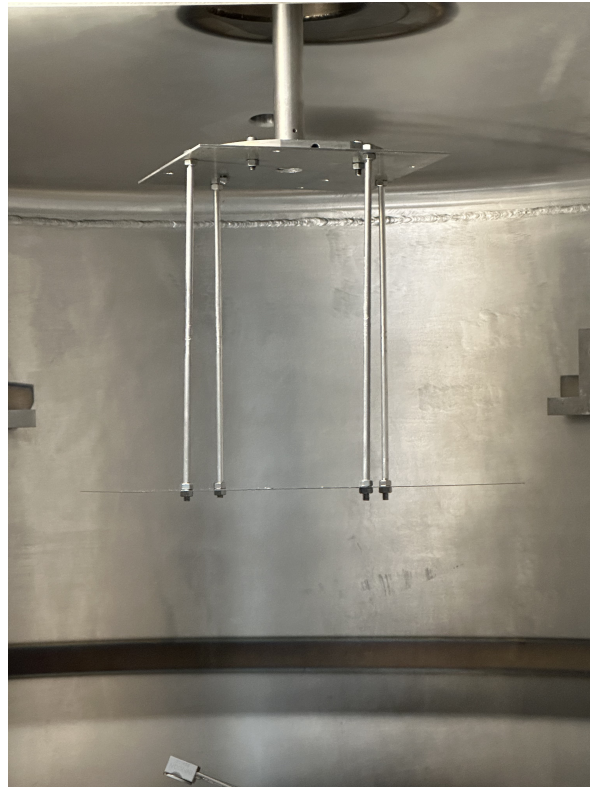
Figure 5: Shows the new mounting scheme, at the bottom of which samples would be taped or clamped onto.
