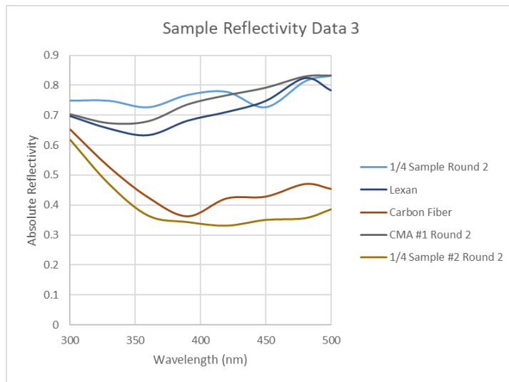
Figure 16: Portrays the reflectivity of the third set of samples, ranging from 300-500 nm wavelength \pm 2 nm.
