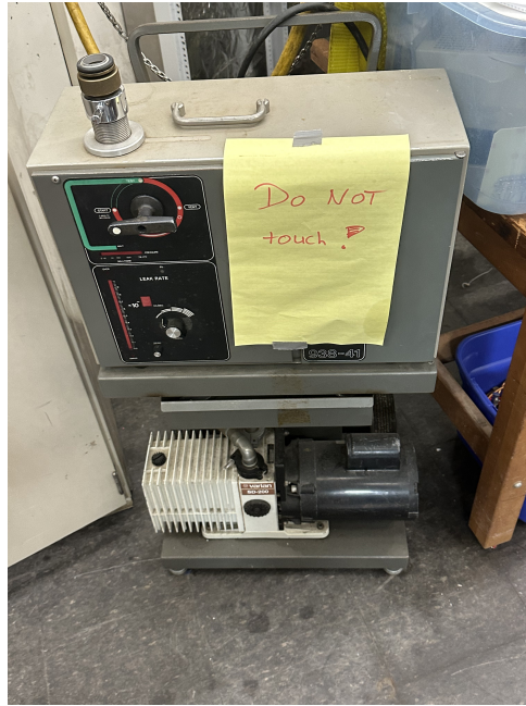
Figure 3: The image shows the existing Varian Leak Detector, despite requiring repairs and servicing it appeared to be a likely candidate to use for testing the connections.
