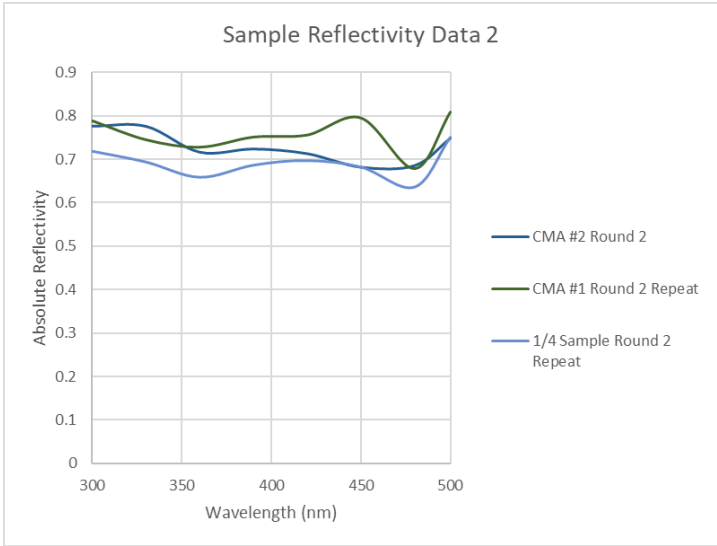
Figure 15: Portrays the reflectivity of the second set of samples, ranging from 300-500 nm wavelength \pm 2 nm
