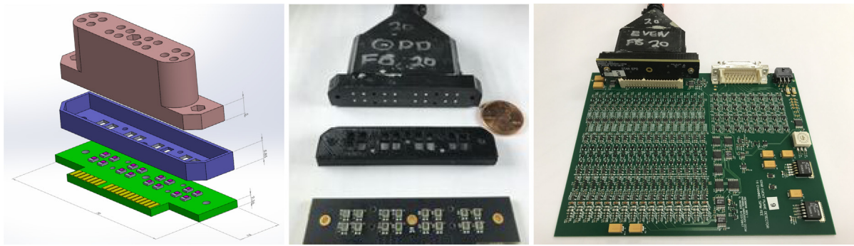
Fig. 4. On the left is a schematic of the FSC connector, the spacer, and the SiPM board. In the middle is a picture of the same assembly, with a penny for scale. The shields, connecting funnel and protective black tubing can also be seen. On the right is the assembly plugged into the FEE board.
