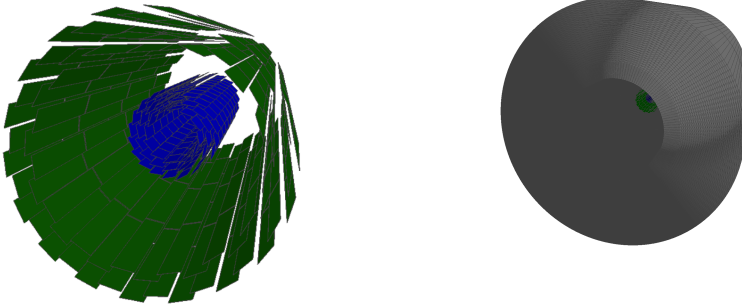
Figure 2. (left) A 3D rendering of the sPHENIX silicon detectors as implemented in ACTS. The small blue layers are the MVTX, and the large green layers are the INTT. (right) A 3D rendering of the sPHENIX TPC layers as implemented in ACTS. Surfaces are created in place of the TPC pad rows to form cylindrical approximations of the TPC. The MVTX and INTT layers can be seen within the inner TPC layer.
