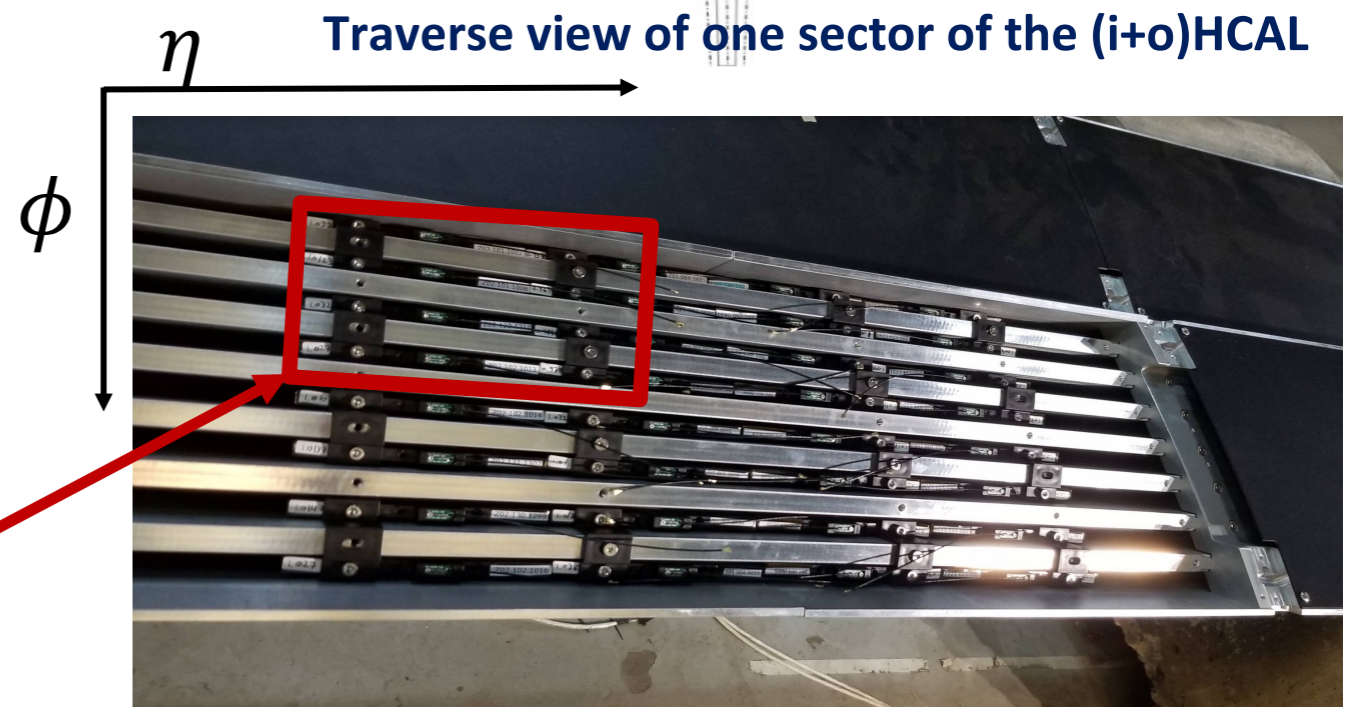
A section of iHCAL sector with tiles and SiPMs
