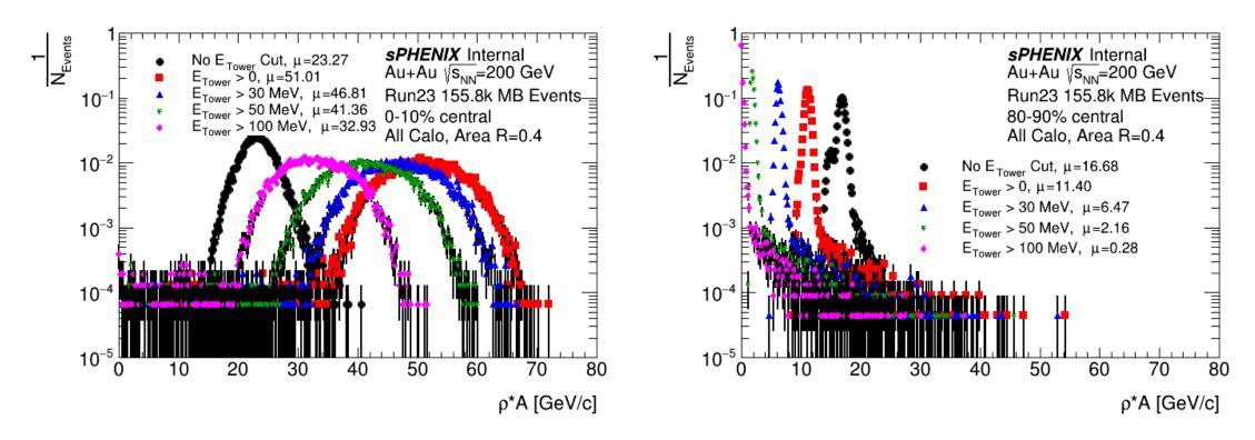
Threshold has large effect on CEMC, which effects total when using all calos
