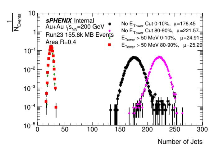
The explanation for a changing number of jets can be seen here, with the number of jets significantly dropping with a tower energy cut implemented
