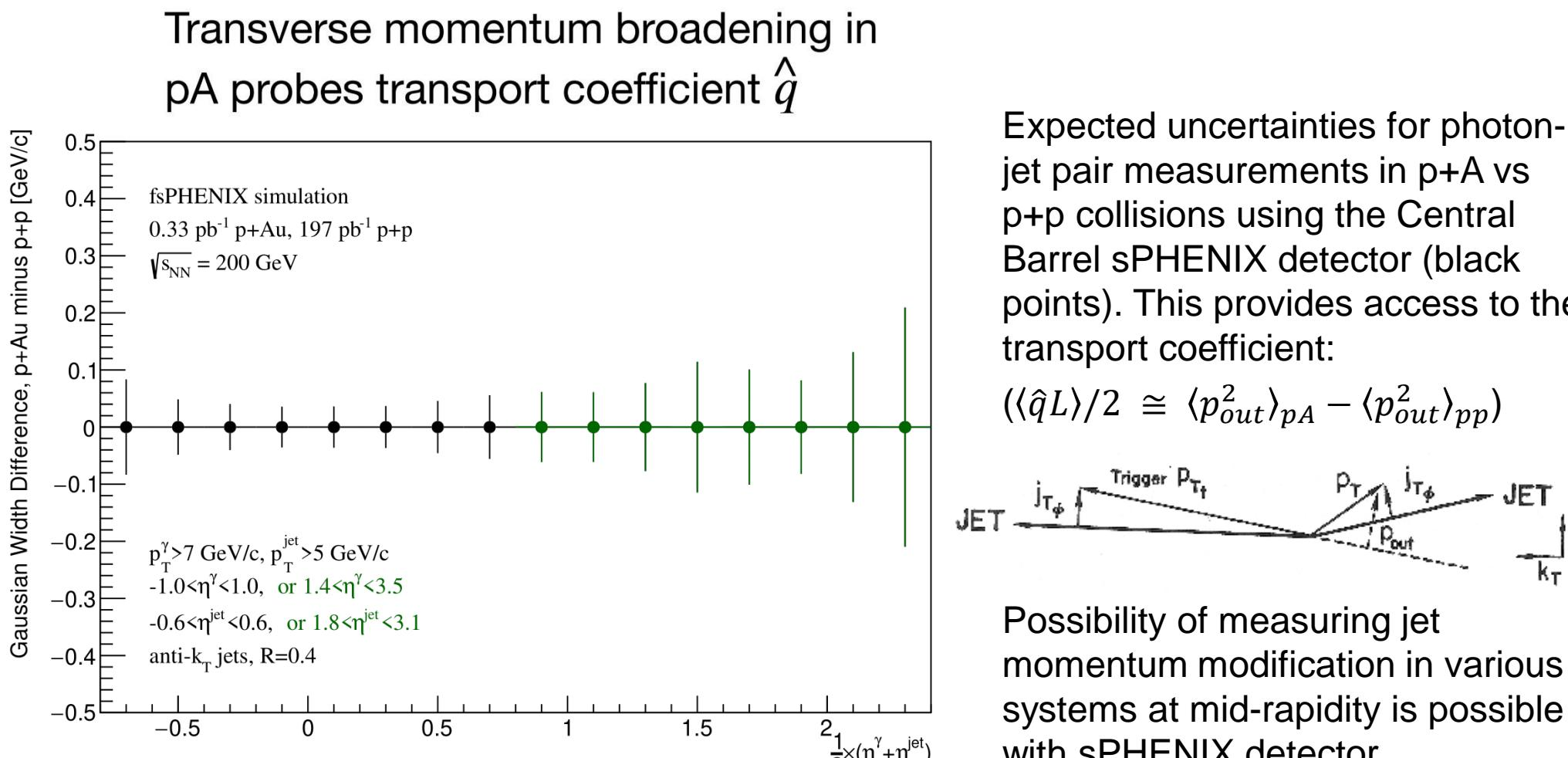
Expected uncertainties for photon-jet pair measurements in p+A vs p+p collisions using the Central Barrel sPHENIX detector (black points). This provides access to the transport coefficient:
