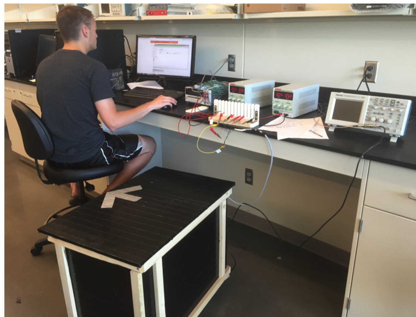
Figure 3: Test bench with dark box and the bench with power supplies for the SiPM and preamp.
