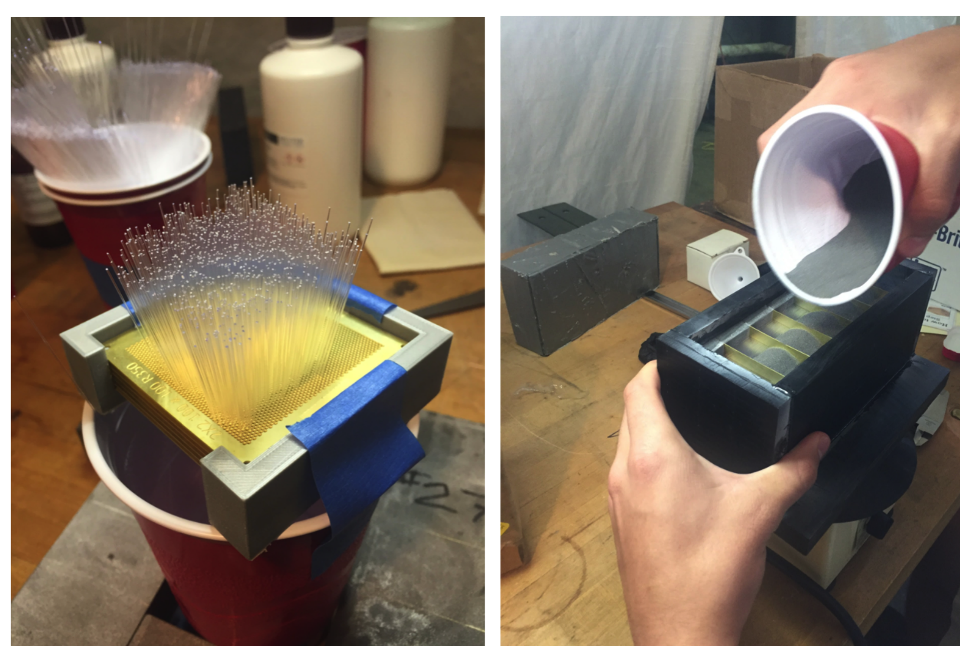
Figure 5: Left: Filling scintillating fibers that are projective in two dimensions. Right: Filling tungsten powder. Epoxy will be poured over the tungsten to produce the modules.
