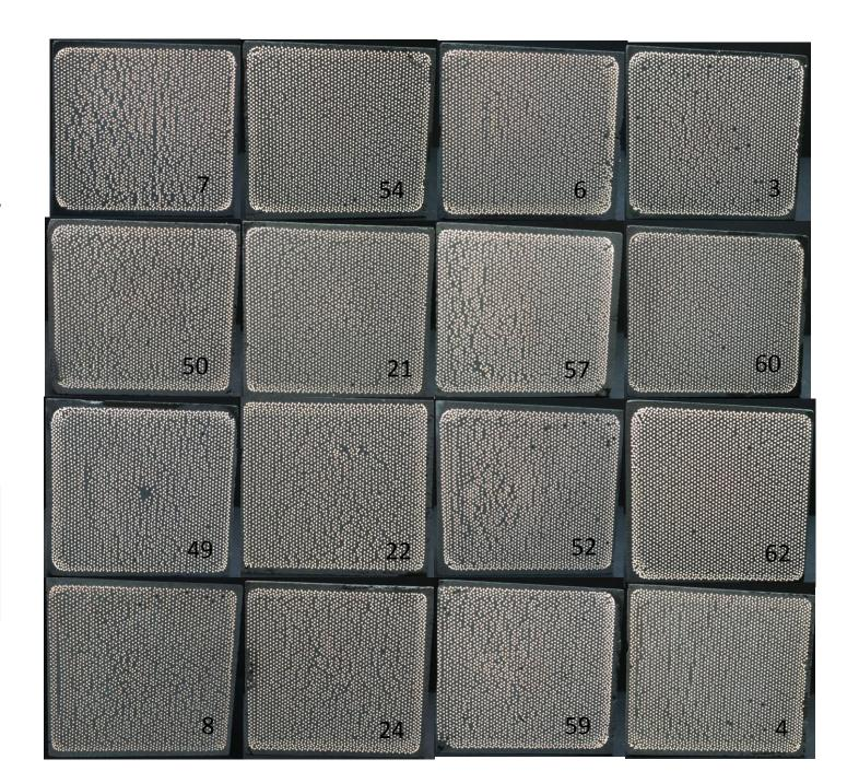
This is how the blocks were Arranged in the V2.1 Prototype (view from back, looking upstream)
