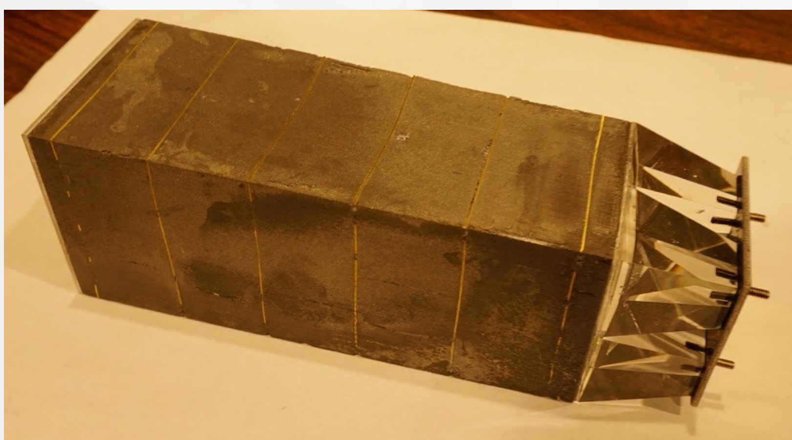
Block with reflector, light guides and SiPMs mounted
