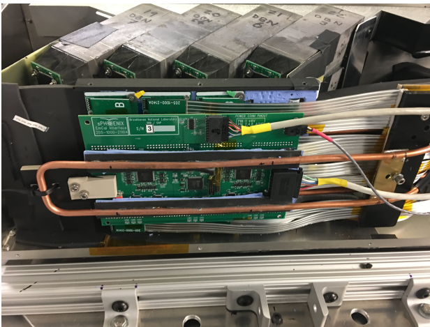
Fig. 4. EMCAL prototype showing the SciFi/W blocks, lightguides, SiPMs, electronics and part of the cooling system.
