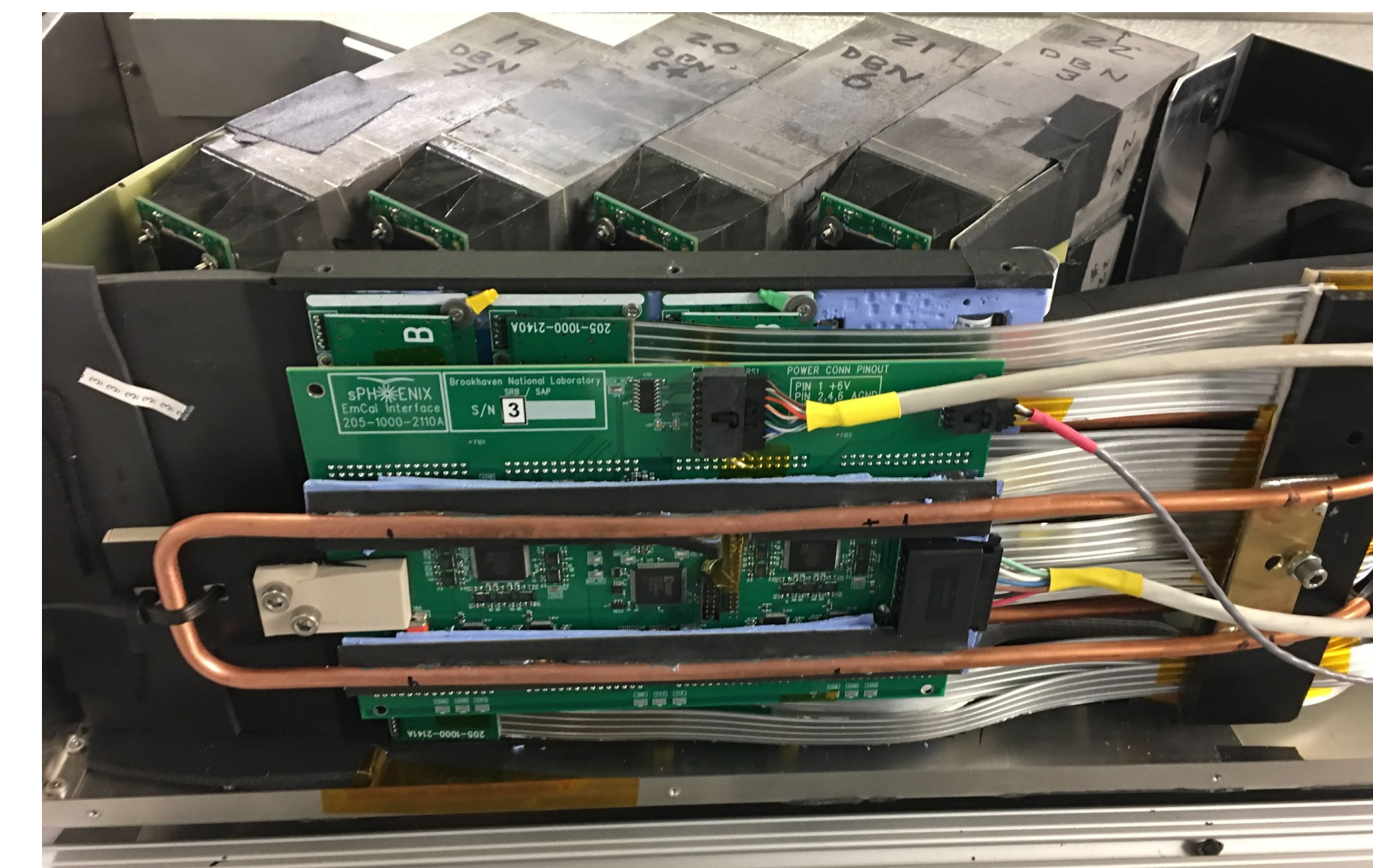
Picture of the EMCAL prototype showing the blocks, light guides, SiPMs, electronics and part of the cooling system.
