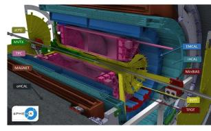
EMCal consists of 64 sectors (32 azimuthal × 2 longitudinal)
