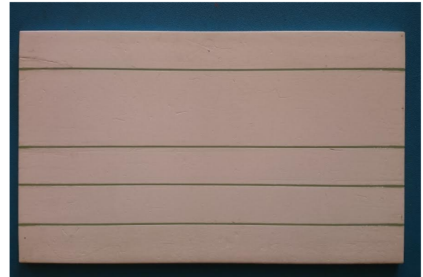
A1 - Panel with diffusive coating (old)
