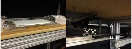
We have both phototubes under the table so that source/LED scans can be run without total deconstruction
