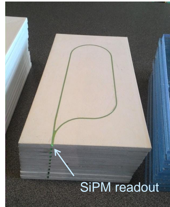
Scintillating tiles with WLS fiber in groove. One SiPM reads out both ends of fiber.
