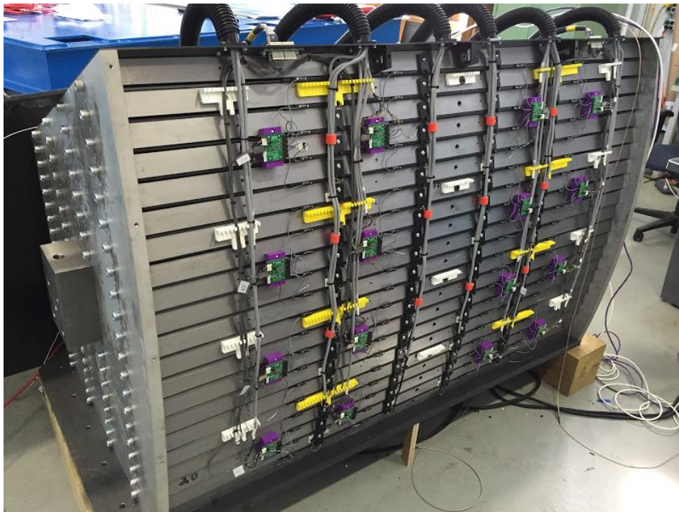
Outer HCAL prototype with assembled steel plates
