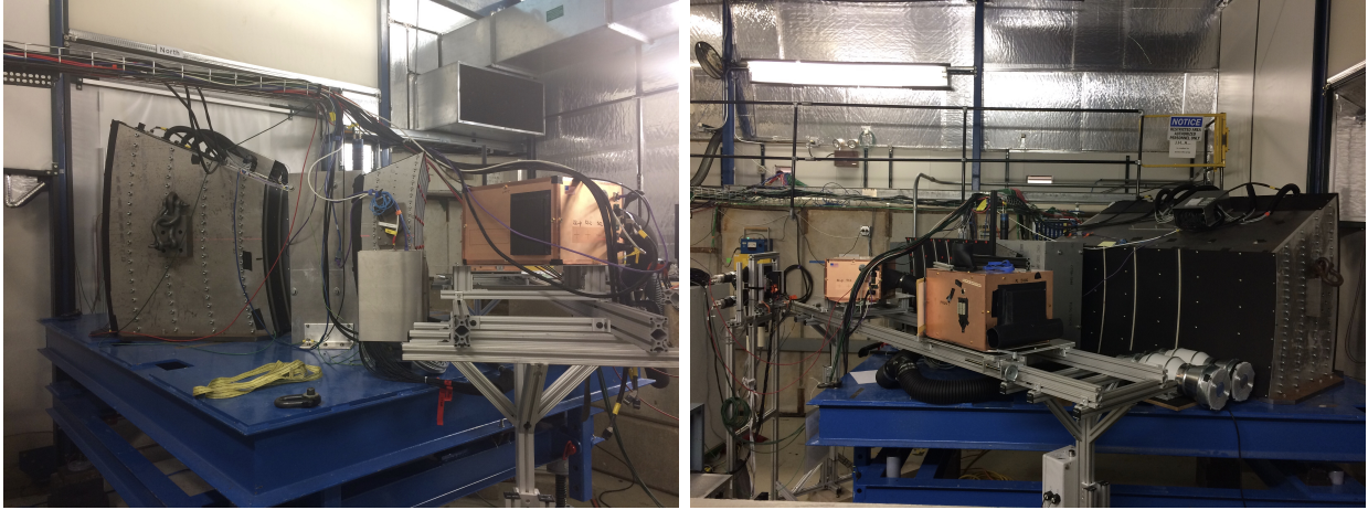
Figure 1: Photographs of the T-1044 setup in 2017. The left plot shows a closeup of the calorimeter system, and upstream is to the right. The right plot shows a slightly zoomed out version where upstream is to the left.
