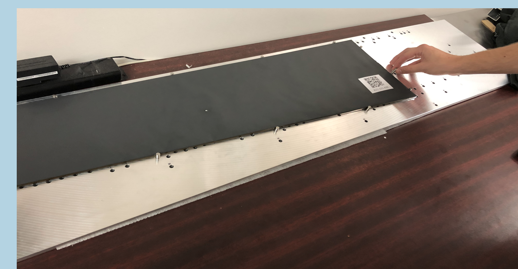
Dimension tester, where tiles are tested to make sure they are the proper size and will fit in the Hcal towers.
