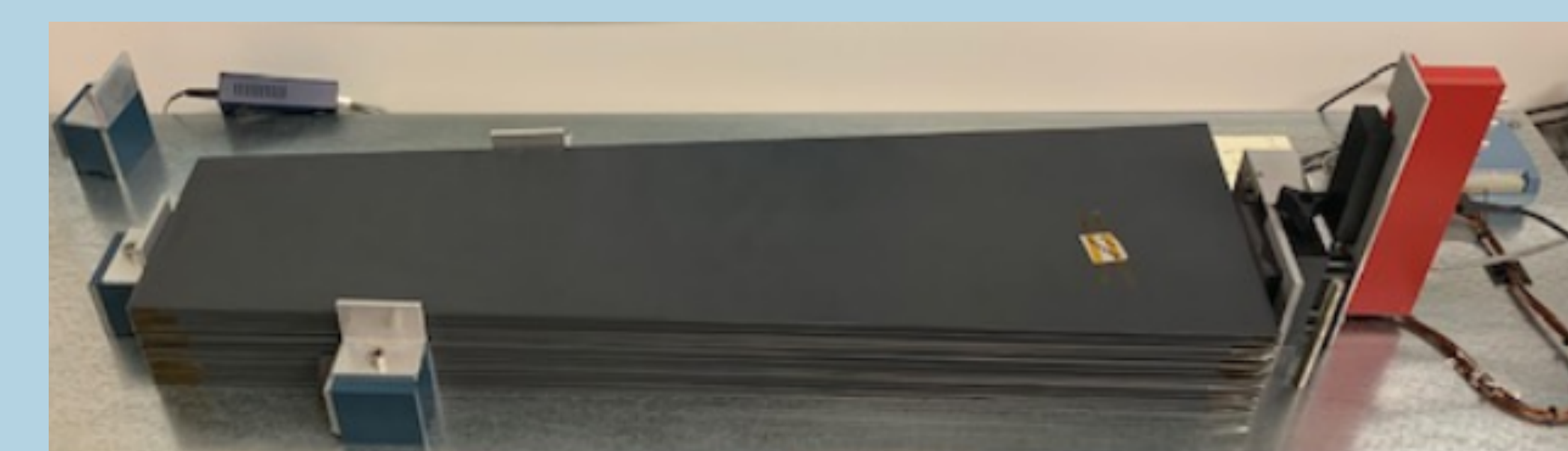
Tile test stand, where 10 tiles (2 reference) are tested for 20 minutes.
