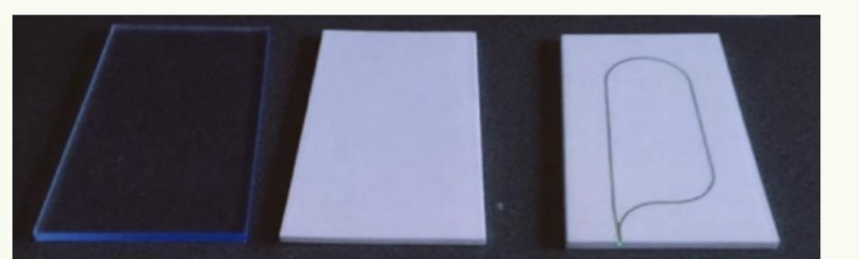
Inner HCal tile composition: Scintillating plastic (left); Reflective coating (middle); Bonded wavelength shifting fiber (right).
