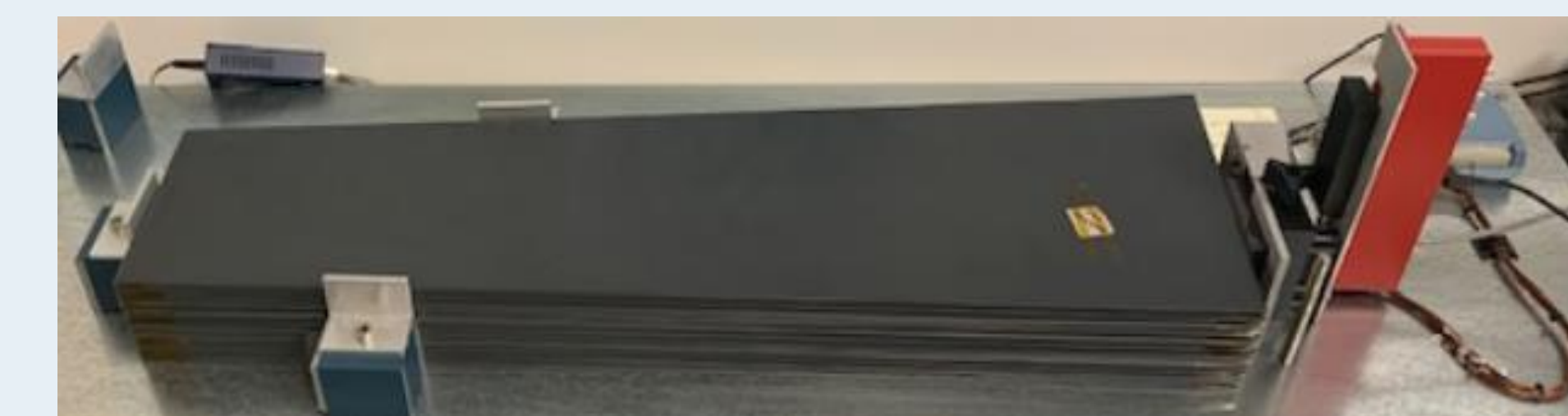
Tile test stand. 10 tiles (2 reference) are tested for 20 minutes.
