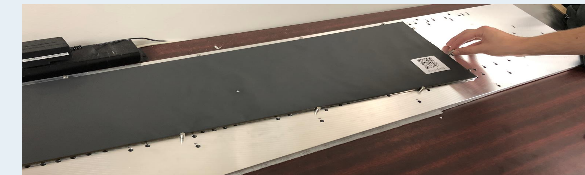
Dimension tester. Tiles are tested to make sure they are the proper size and will fit in the HCal towers.
