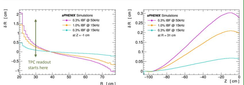
The top (bottom) plots show the distortion in the radial (phi) direction in the regions where the distortion is maximal. For the Ne-based gases and setup under consideration, the expected distortions are below 2 cm at 15kHz and 3 cm at 50 kHz. (for the effect of distortions on tracking, see Sourav's poster)
