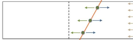
**Ion BackFlow (IBF)** from the GEM stage is also a source of SpaceCharge. For high rate data acquisition, IBF is the main source of SpaceCharge buildup.
