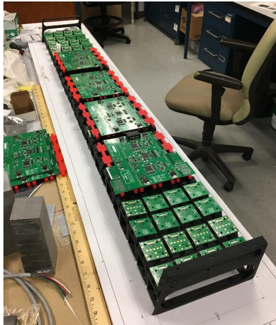
Figure 2. Mockup of the EMCAL preproduction prototype made from 3D printed parts with mockup parts of the cooling system (red) and prototype readout electronics installed.
