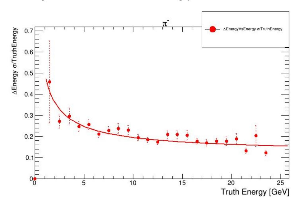
For matched topoclusters to generated  $\pi^-$ ,  $\sigma_E/E_{True}$  shows better than 20% energy resolution above 10 GeV and consistent with sPHENIX test beam data.
