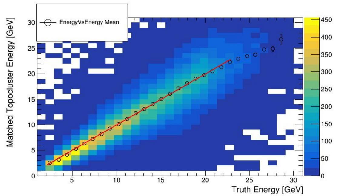
$\pi^-$  matching topocluster energy levels to their corresponding truth particle after calibrating the slope to approximately 1. The slope is 0.996 +/- 0.0026.
