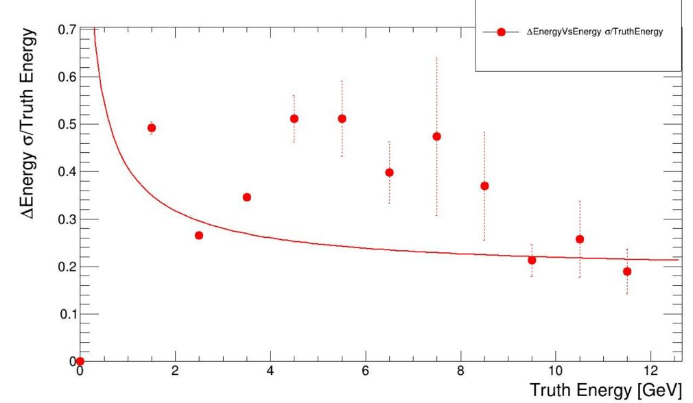
For isolated topoclusters matched to truth particles,  $\sigma_{\rm F}/E_{\rm True}$  shows resolution similar to single particles.
