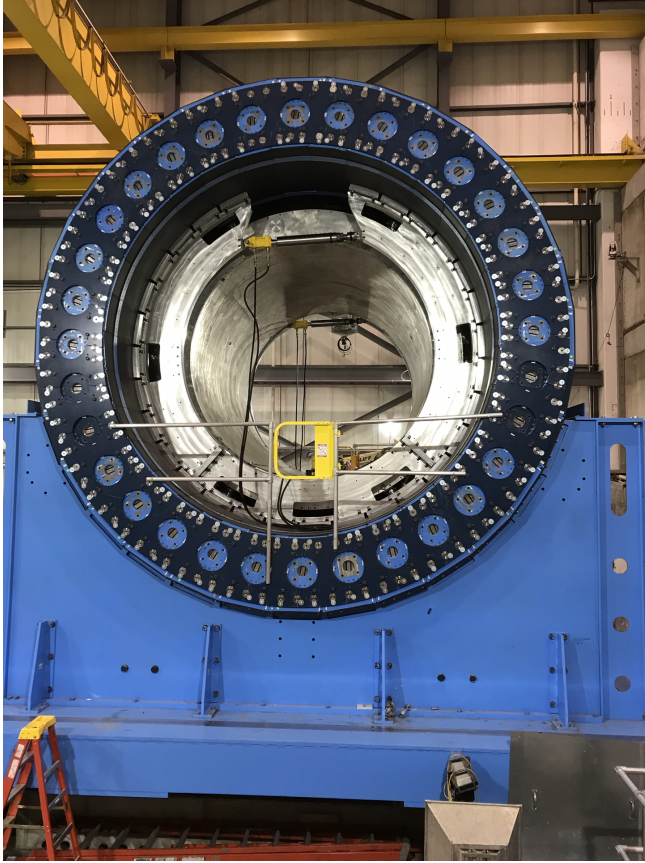
FIGURE 8. Outer Hadronic Calorimeter completely assembled and installed in the sPHENIX assembly hall at RHIC
