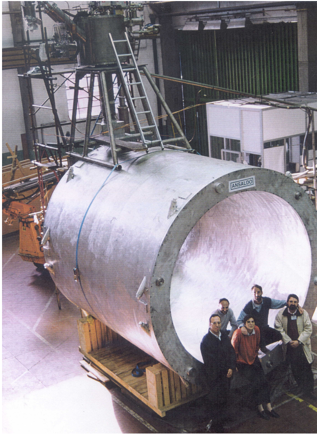
Figure 1.2: The superconducting solenoid after the cryogenic test at Ansaldo (Genova). One can see the annular cryostat enclosing the superconducting solenoid and the turret with proximity cryogenics and current leads.
