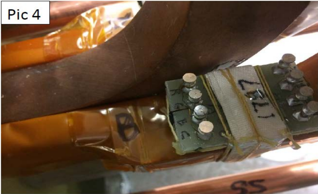
Figure 3: Pictures of the RTD (resistive temperature detectors), “Pic 1” and “Pic 2” and their intended locations on the Cryo Extension, “Pic 3” and “Pic 4”.
