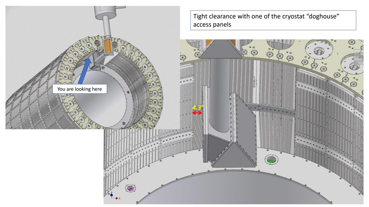
Tight clearance with one of the cryostat "doghouse" access panels
