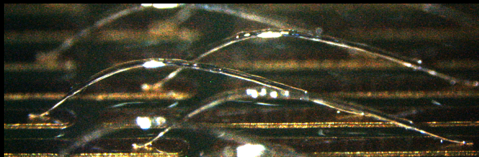
PU light coat \sim 50 \mu O.D.
