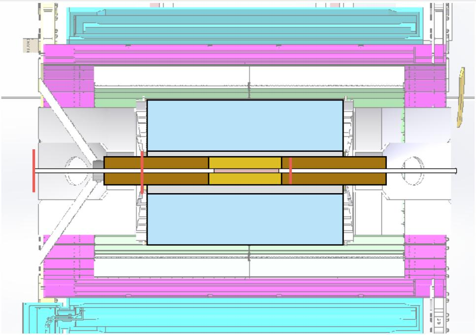
INTT slides in on rails. ROCs do not interfere with support. Internal beampipe guide limits sag.
