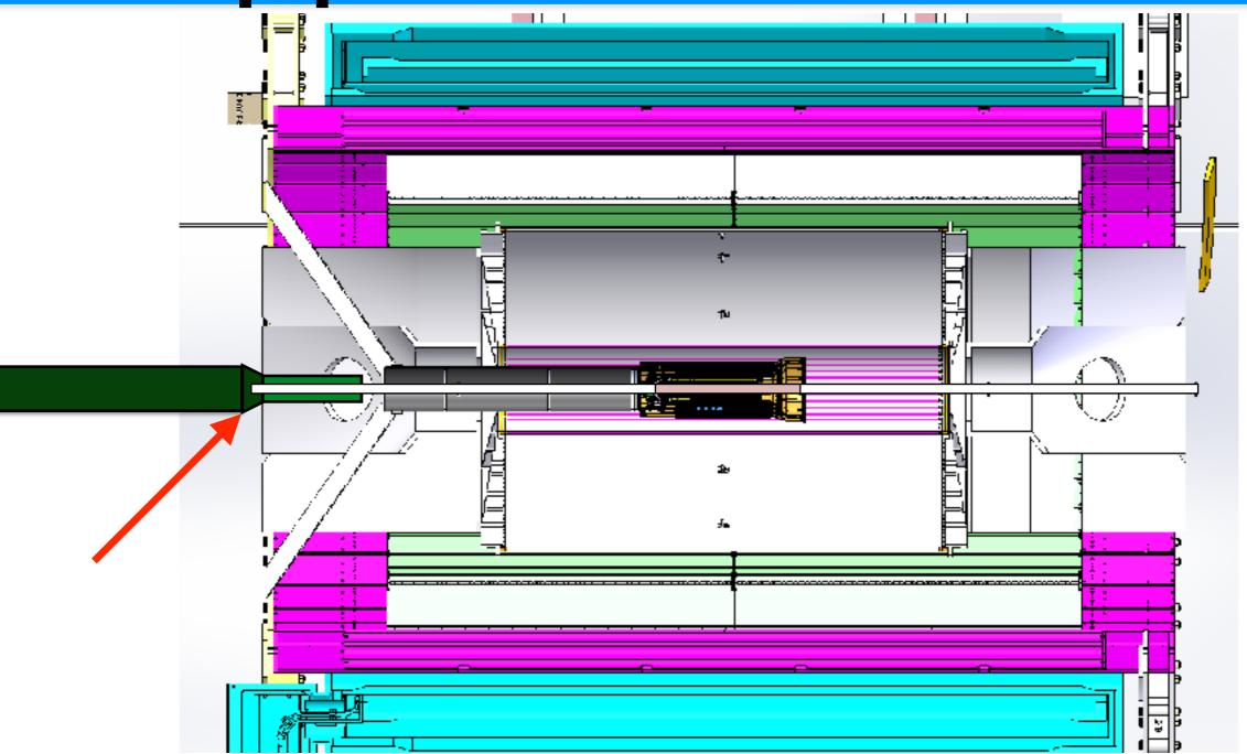
Want flange moved back so MVTX can clamshell outside of TPC bore before insertion. Beampipe
