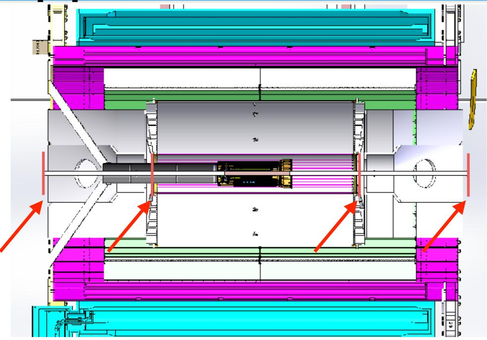
Symmetric extension causes sag >2mm if pipe unsupported, so use supports at flanges and TPC wagon wheels
