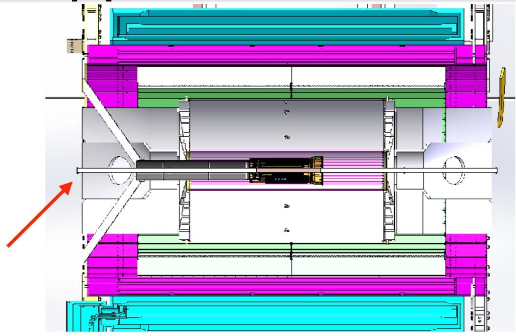
Want flange moved back so MVTX can clamshell outside of TPC bore before insertion. Beampipe
