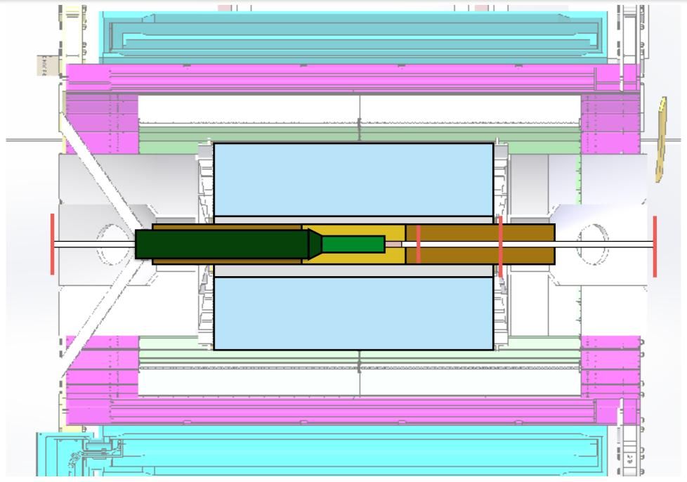
South TPC support removed, MVTX slides in, buttons up past flange support.
