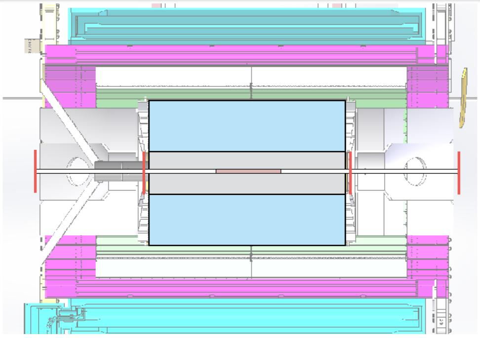
TPC, INTT rails, beampipe, and temporary supports installed
