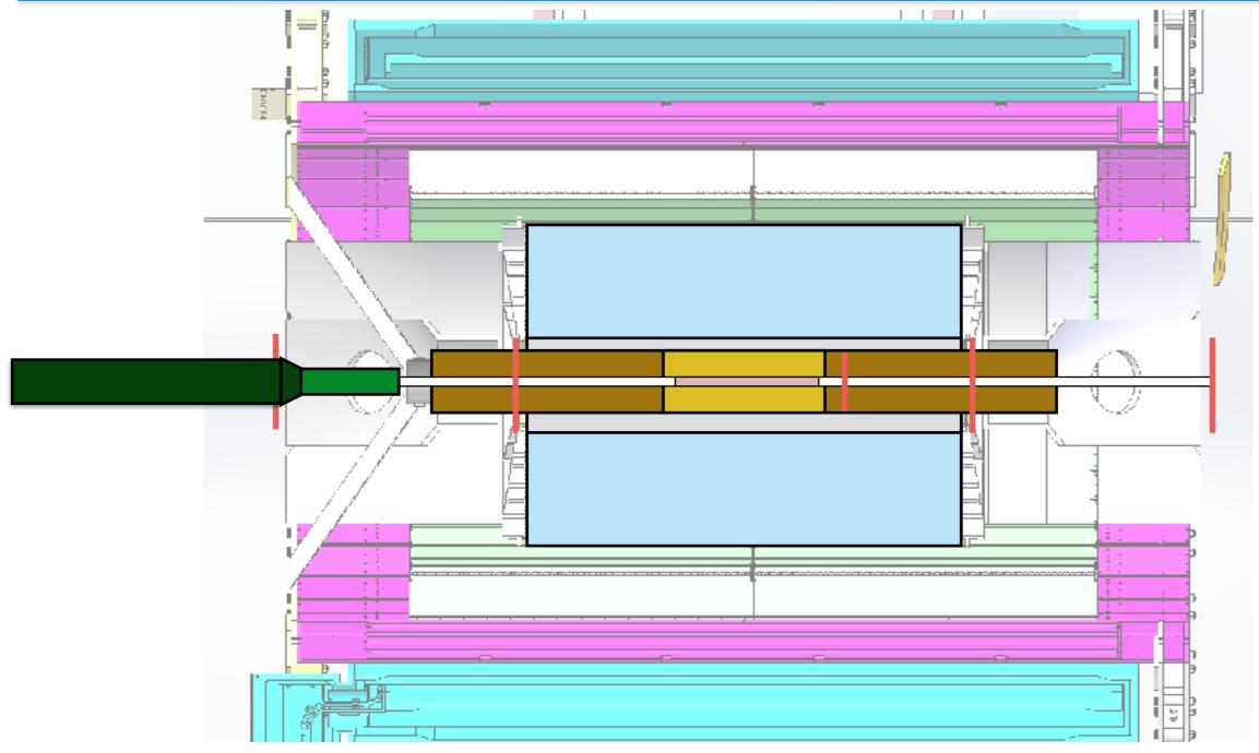
MVTX support installed, MVTX installed north of flange. Barrel has gap for flange support.
