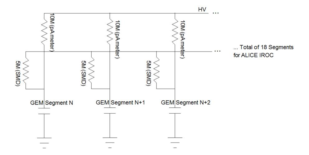
For a given IROC segment a simplified circuit is shown. One is interested in the current through the GEM segment resistance shown in red.
