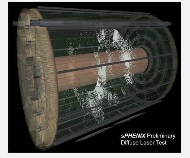
• Hits in TPC from test laser flash shows clear indication of CM stripe pattern and sheets of electrons
