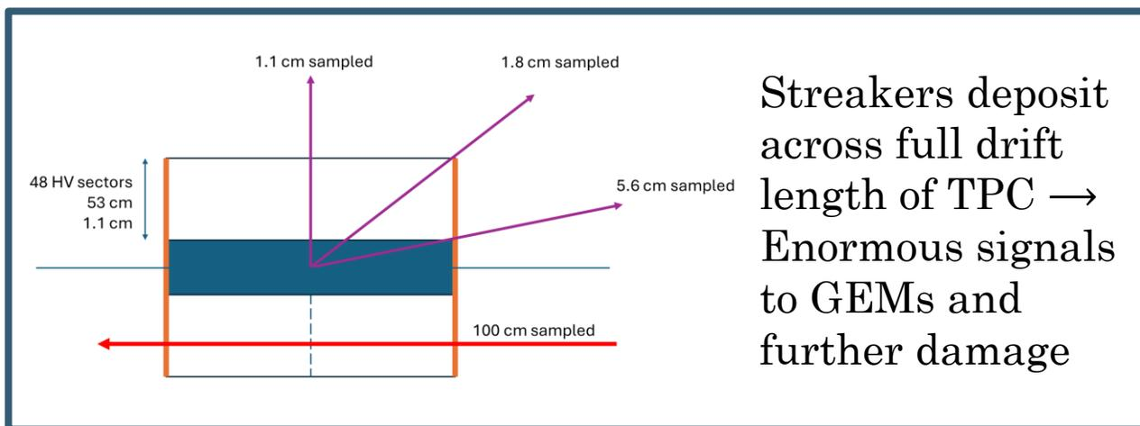
Streakers deposit across full drift length of TPC → Enormous signals to GEMs and further damage
