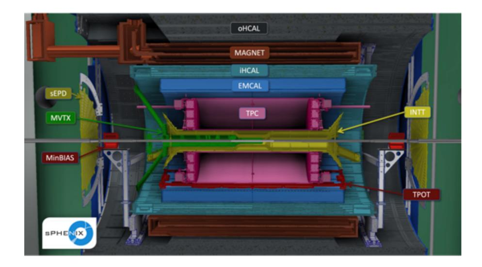
The sPHENIX tracker (1.4 T magnetic field) consists of:
