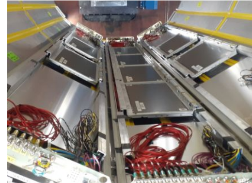
TPOT assembly structure
