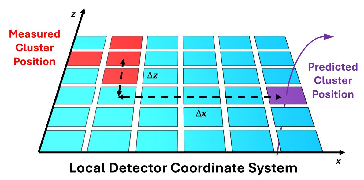
Residual = (Measured Cluster Position) – (Intersection of Track Fit with Physical Detector Surface)
