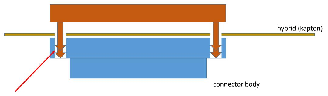
Secure the "posts" into former screw holes in connector body using some epoxy. Of course, done *after* the connector soldering.
