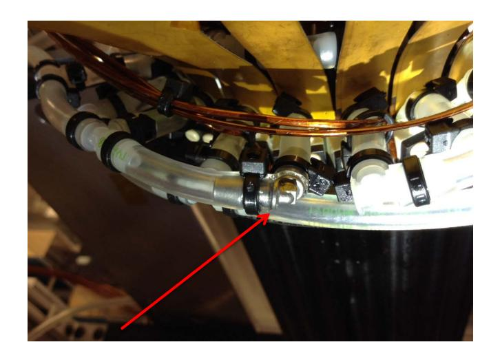
Location of leaking fitting. East detector, barrel 1. South Side. Bottom loop. Fitting was a plastic elbow. Leak was confirmed with a sniffer and Snoop. The fitting was replaced with a stainless elbow.
