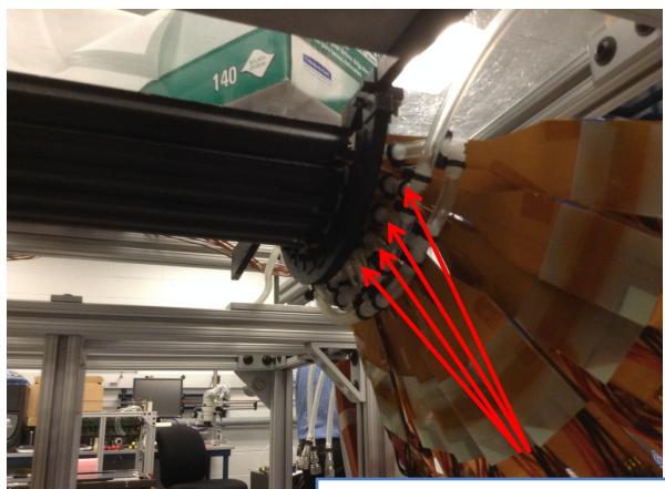
Sniffer indicates more leaks along the base of several B1 staves (top loop, South side— Pressure drops about 10 psi in 15 minuites
