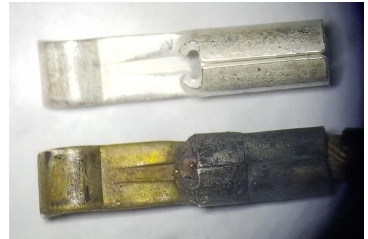
Fig.9 New contact on top Vs contact removed from the field Contact on bottom shows signs of pitting & excessive heating
