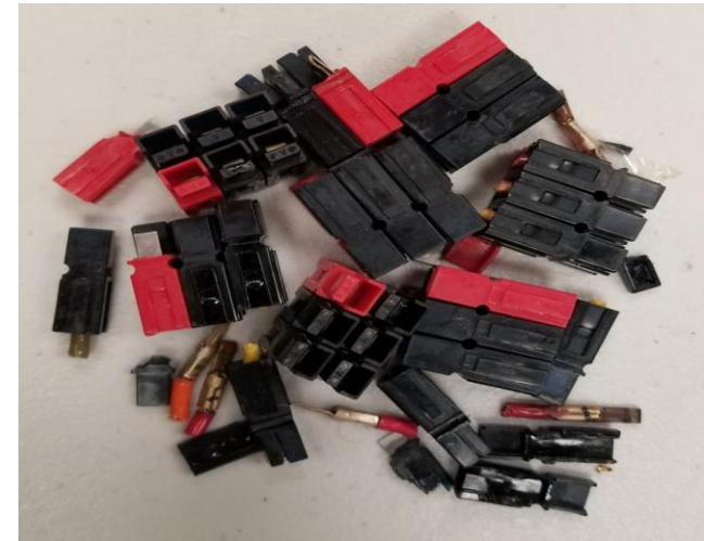
Contact housing & connector removal for typical repair of LV interconnect (parts removed from 4x sectors shown)
